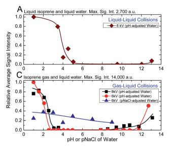
Fig. 3 Influence of the ionic strength and ESI voltage on the ESIMS spectra of experimental sets (A) and (C). On the y-axis, we plot the average mass spectral intensity of all the oligomeric peaks [(Isop) $_n$ ·H] $^+$ , given by  $\sum I_n/n$ , normalized by the highest datum in each plot. (A)
