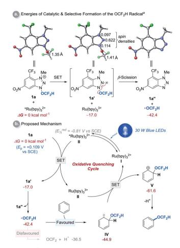
Scheme 3 Computational studies and proposed reaction mechanism. <sup>a</sup>DFT calculations were performed at the M06-2X/6-311++G(d,p)/ SMD(MeCN)//M06-2X/6-31+G(d) level of theory using reagent 1a and benzene as a substrate. All energies are in kcal mol<sup>-1</sup> and are with respect to II and 1a. See (ESI†) for details
