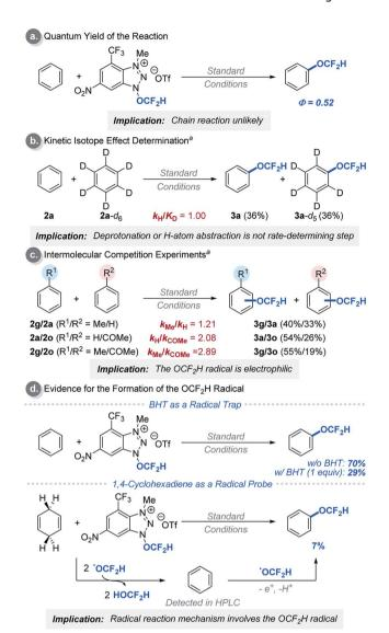
Scheme 2 Experimental mechanism studies: <sup>a</sup>reactions were performed using 5.00 equivalents of arenes each. See ESI† for experimental details.
