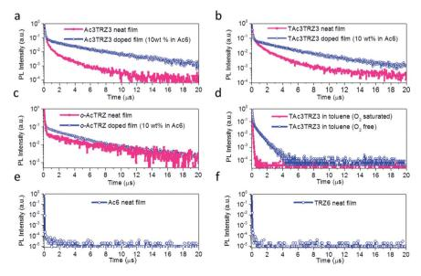
Fig. 4 Transient PL decay of the TSCT-HABs. PL decay curves of the Ac3TRZ3, TAc3TRZ3 and o-AcTRZ in neat or doped films (a–c), TAc3TRZ3 in N<sub>2</sub> or O<sub>2</sub> saturated toluene ( $10^{-5}$  mol L<sup>-1</sup>) (d), and the Ac6 and TRZ6 neat films (e and f).
