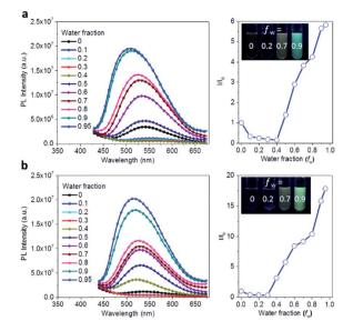
Fig. 5 Aggregation-induced emission effect of the TSCT-HABs. PL spectra and the relative emission intensity of Ac3TRZ3 (a) and TAc3TRZ3 (b) in THF/water mixed solvents at a concentration of  $1 \times 10^{-5}$  mol L<sup>-1</sup>; inset: PL images with different water fractions ( $f_{\rm w}$ ) under UV light (365 nm).
