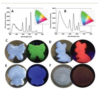
Fig. 6 Emission profiles of Eu–Tb–Dy MOF gels under the single-wavelength excitation at 275 nm with the Eu/Dy/Tb ratios of (A) 1:1:1 and (B) 1:1:2. Photographs of (C) Tb–Dy, (D) Eu–Tb, (E) Eu–Dy, and (F) Eu–Tb–Dy MOF gels with mixed-metal ratios of 1:1 or 1:1:1 under sunlight (left) and excitation at 275 nm (right).
