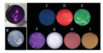
Fig. 7 (A) UV torch with excitation at 275 nm. (B) The photo of MOF gels coated on the torch under sunlight. The emission of MOF gels coated on the torch with different types and ratios of  $Ln^{3+}$  ion of (C) Dy, (D) Eu/Tb of 1:1, (E) Tb/Dy of 1:1, (F) Eu/Dy of 1:1, (G) Eu/Tb/Dy of 1:1:2, (H) Eu/Tb/Dy of 2:1:1, (I) Eu/Tb/Dy of 1:2:1 after the torch was lit
