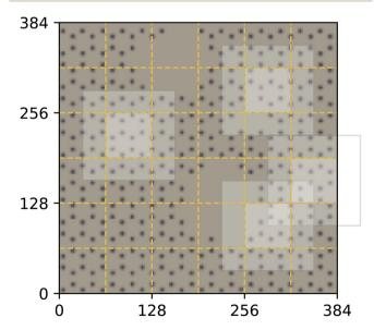
Fig. 4 Decomposition of input image for the quantum mechanical density functional theory calculation using f = 64 and c = 32. Four tiles consisting of a focus region and context region are highlighted. Overlap in the context region is by design and the EDNN must learn to ignore this overlap in the final reduction of the extensive quantity.
