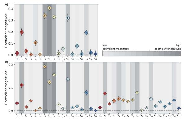
Fig. 4 Coefficient magnitude distributions of the input features of the trained (A) BNN1 and (B) BNN2. Input features {r<sub>i</sub>} and {v<sub>i</sub>} correspond to geometry coordinates and velocities along normal modes, respectively. The numbering of the normal modes goes from 0 to 17, 0 being the reaction coordinate
