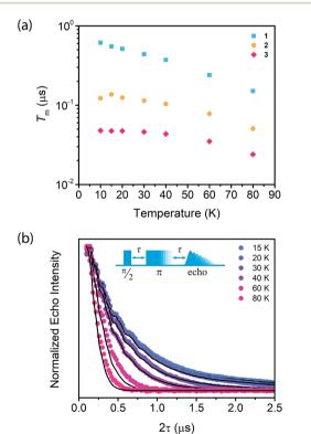
Fig. 2 (a) Temperature dependence of  $T_{\rm m}$  of 1, 2, and 3, collected at 3328 G for 1 and 2 and at 3410 G for 3 from 10–80 K. The Hahn Echo pulse sequence used to measure  $T_{\rm m}$  is shown at the bottom. (b) Representative fits to the Hahn echo decay of 1 at 2942 G across 15–80 K based on our model incorporating electron–electron spin distances and  $T_{\rm 1}$ .
