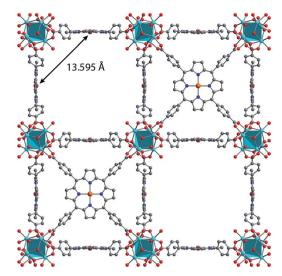
Fig. 1 Crystal structure of the new material Cu<sub>1.0</sub>-PCN-224 (3) with each porphyrinic ligand metalated with Cu<sup>2+</sup>. Orange, red, blue, and gray represent copper, oxygen, nitrogen, and carbon, respectively. [Zr<sub>6</sub>O<sub>6</sub>] nodes are represented by the turquoise polyhedra. Nearest neighbor distances between Cu<sup>2+</sup> centers are highlighted.
