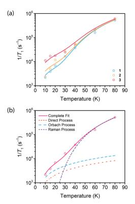
Fig. 4 (a) Fits to the temperature dependence of  $1/T_1$  for 1, 2, and 3 at 3328 G. Results of the fits are reported in Table S13.† (b) Fit to the temperature dependence of  $1/T_1$  of 1 at 3328 G resonance. The red line represents the total fit, while the orange, blue and purple dashed lines represent the contributions of the direct, Orbach–Aminov and Raman processes, respectively.
