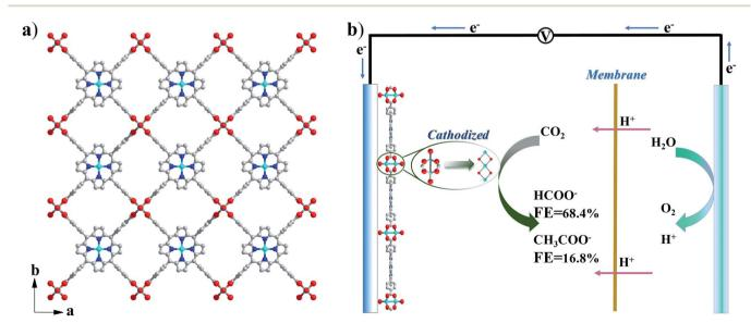
Scheme 1 (a) Crystal structure of  $Cu_2(CuTCPP)$  nanosheets along the c axis. Red is O, blue is N, grey is C and cyan is  $Cu_2(CuTCPP)$  nanosheets along the c axis. Red is O, blue is N, grey is C and cyan is  $Cu_2(CuTCPP)$  nanosheets along the c axis. reduction system with Cu<sub>2</sub>(CuTCPP) nanosheets as the catalyst.
