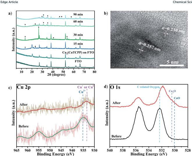
Fig. 4 (a) XRD of Cu<sub>2</sub>(CuTCPP) nanosheets on a FTO electrode with different reaction times (● Cu(HCOO)<sub>2</sub>; ◆ Cu<sub>4</sub>O<sub>3</sub>; ▲ Cu(OH)<sub>2</sub>; ▼ CuO; ★ Cu<sub>2</sub>O); (b) HRTEM after 5 h reaction; (c) Cu 2p XPS spectra and (d) O 1s XPS spectra of Cu<sub>2</sub>(CuTCPP) on FTO before and after 5 h reaction. All potentials were set at -1.55 V vs. Ag/Ag<sup>+</sup>.
