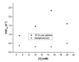
Fig. 5 Dependency of the  $TOF_{ini}$  on the substrate concentration at constant ratio [1]/[Et<sub>3</sub>N], when the <code>XantphosCu(i)</code> (red dots) is used or when 12 <code>SXantphosCu(i)</code> in the nanosphere are applied as the catalyst (black square). For reaction conditions see ESI Fig. S53†
