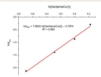
Fig. 2 Dependence of the  $k_{\rm obs}$  of the cyclization of 4-pentynoic acid with the concentration of XantphosCu(i) (kobs obtained from Fig. S44 in the ESI+).
