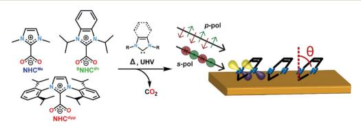
Fig. 1 Schematic showing the molecular structure of the NHC precursors, the thermal decomposition/sublimation deposition approach to create the NHC monolayers, and the NEXAFS dichroism measurement. Free NHC molecules are generated in the gas phase upon heating.
