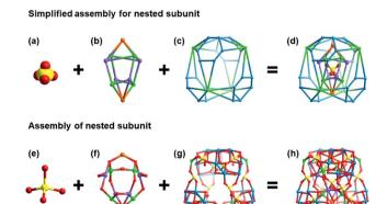
Fig. 1 Simplified (a–d) and real (e and h) three-shell nested subunit for NENU-605. (a, e) The innermost shell (central  $PO_4^{3-}$  group); (b, f) the shuttle-shaped second shell ( $\{Na_2K_4Mn_4\}\}$ ; (c, g) the cage-like outermost shell ( $\{Mn_4(\{P_4Mo_6\}\}_4\}$ ; (d, h) the overall three-shell nested substructure. Colour code: P yellow, O red, Na orange, K light purple, Mn green, and Mo light blue.
