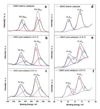
Fig. 10 Pd 3d XPS spectrum of 1|NiO (a) before photoelectrocatalysis, after photoelectrocatalysis under (b)  $E_{\rm appl} = -0.4~{\rm V}$  and (c)  $E_{\rm appl} =$ -0.6 V; Pt 4f XPS spectrum of 2|NiO (d) before photoelectrocatalysis, after photoelectrocatalysis under (e)  $E_{appl} = -0.4 \text{ V}$  and (f)  $E_{appl} =$ -0.6 V vs. Ag/AgCl.
