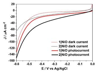
Fig. 6 Linear sweep voltammograms of 1|NiO and 2|NiO immersed in aqueous 0.1 M KCl electrolyte (pH 3). The potential was swept from  $E_{\rm appl} = 0$  to -0.6 V vs. Ag/AgCl (3.0 M NaCl) in the dark and under simulated light illumination (AM1.5, 100 mW cm<sup>-2</sup>).
