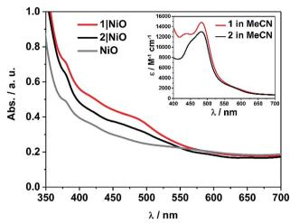
Fig. 2 UV-vis absorption spectra of 1 (red) and 2 (black) adsorbed on NiO and bare NiO (gray). Inset: UV-vis absorption spectra of 1 (red) and 2 (black) in MeCN (0.028 mM and 0.032 mM, respectively).
