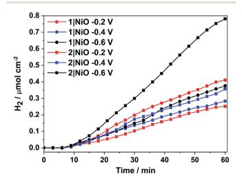
Fig. 8 Cumulative photoelectrocatalytic H<sub>2</sub> production by 1|NiO and 2|NiO during the chronoamperometry measurements at different  $E_{appl}$ (Fig. 7 and S3 in the ESI†). Chopped light illumination was applied during the first 10 min followed by constant light illumination until the end of the measurement (AM1.5, 100 mW cm $^{-2}$ ).
