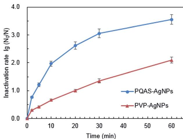
Fig. 2 Inactivation efficiency of *B. subtilis* by PQAS-AgNPs and PVP-AgNPs. Reaction conditions: [AgNPs] = 10.0 mg L<sup>-1</sup>, pH = 7.1, T = 25 °C, initial concentration of bacteria: 10<sup>6</sup> CFU mL<sup>-1</sup>.
