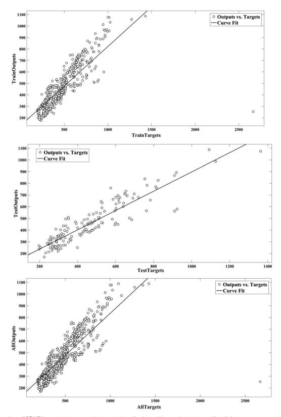
Fig. 5 Scatter plots of PDNFM<sub>SVM</sub> outputs *versus* the target values for the training and test sets and for all data.
