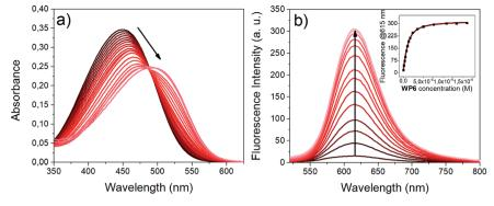
Fig. 3 Complexation of i1 with WP6 in HEPES buffer (pH 7.4). (a) Absorption spectra (10.0  $\mu$ M i1, 0 to 1.74 equiv. WP6) (b) fluorescence spectra (1.0  $\mu$ M i1, 0 to 16 equiv. WP6,  $\lambda_{ex}$  (isosbestic point): 482 nm). The inset shows the fluorescence emission at 615 nm vs. WP6 concentration (black dots: experimental data, red curve: result of non-linear fitting).
