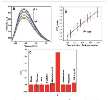
Fig. 7 (a) Fluorescence restoration of CD-Fe<sup>3+</sup> system *via* the addition of ascorbic acid. (b) Relative fluorescence response of CDs-Fe<sup>3+</sup> system  $(F/F_0)$  with different concentrations of AA, (c) fluorescence response of CDs-Fe<sup>3+</sup> system in presence of various biomolecules.
