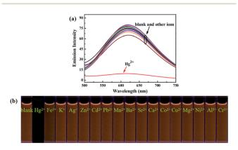
Fig. 7 (a) Fluorescence spectra of luminogen 1 ( $2.0 \times 10^{-5}$  mol L $^{-1}$ ) towards various cations including Zn $^{2+}$ , Cd $^{2+}$ , Hg $^{2+}$ , Ba $^{2+}$ , Sr $^{2+}$ , Mn $^{2+}$ , Mg $^{2+}$ , Ca $^{2+}$ , Pb $^{2+}$ , Ni $^{2+}$ , Co $^{2+}$ , Cu $^{2+}$ , Al $^{3+}$ , Fe $^{3+}$ , Cr $^{3+}$ , Ag $^{+}$  and K $^{+}$ . Excitation wavelength = 380 nm. (b) Fluorescence photographs of luminogen 1 after addition of various metal ions (7.0 equiv.) under 365 nm light.
