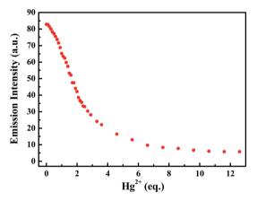
Fig. 5 The emission intensity changes of luminogen  $\bf 1$  at 625 nm with different equivalents of  $Ha^{2+}$ .
