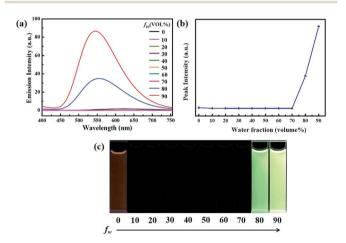
Fig. 1 (a) Fluorescence spectra of the dilute solutions of 1 (2.0  $\times$   $10^{-5}$  mol L $^{-1}$ ) in acetonitrile–water mixtures with different water content (0–90%). Excitation wavelength = 380 nm. (b) Changes the emission intensity of 1 at 545 nm in acetonitrile–water mixtures with different volume fractions of water (0–90%). (c) PL images of 1 (2.0  $\times$   $10^{-5}$  mol L $^{-1}$ ) in acetonitrile–water mixtures with different  $f_{\rm W}$  values under 365 nm UV illumination.
