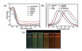
Fig. 3 (a) UV-Vis absorption spectra and (b) normalized fluorescence spectra (Excitation wavelength =380 nm) of luminogen 1 in different solvents (2.0  $\times$   $10^{-5}$  mol L $^{-1}$ ). (c) Photographs of 1 under 365 nm UV illumination in different solvents: tol (toluene); THF (tetrahydrofuran); EA (ethyl acetate); BT (acetone); MeCN (acetonitrile); DMSO (dimethyl sulfoxide).
