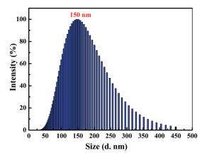
Fig. 2 Size distribution curve of luminogen 1 (2.0  $\times$  10<sup>-5</sup> mol L<sup>-1</sup>) in acetonitrile—water mixtures with  $f_{\rm w}=90\%$ .
