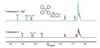
Fig. 6  $^{1}$ H NMR (acetonitrile- $d_{3}$ , 400 MHz) spectra changes of luminogen 1 in the presence of Hg<sup>2+</sup>.
