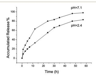
Fig. 2 IBU release processes from the HMMS system in a neutral solution (pH 7.1) and an acidic solution (pH 2.4).<sup>56</sup>
