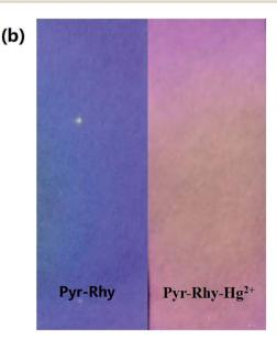
Fig. 9 Photographs showing the color changes of sensor Pyr-Rhy before and after addition of Hg<sup>2+</sup> under (a) sunlight and (b) 365 nm UV light.
