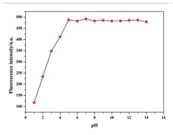
Fig. 6 Effect of pH on the fluorescence intensity of sensor Pyr-Rhy toward Hg<sup>2+</sup> in DMSO/H<sub>2</sub>O (1/1, v/v) solution.
