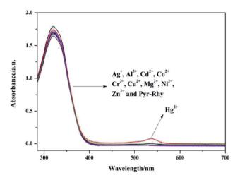
Fig. 2 UV-vis absorption spectra of sensor Pyr-Rhy (10  $\mu$ M) upon addition of different metal ions (10  $\mu$ M) in DMSO/H<sub>2</sub>O (1/1, v/v) solution.
