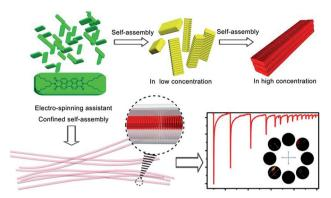
Scheme 1 Schematic representation for the hierarchical assembly in solid-state and electro-spinning assistant confined self-assembly of N,N'-bis(1-hexylheptyl)perylene-3,4,9,10-tetracarboxylbisimide (PDI) for optical sensing applications.
