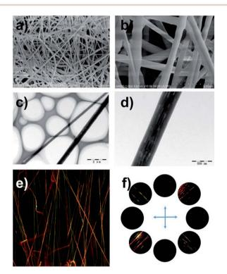
Fig. 2 (a) SEM (scale bar =  $20 \mu m$ ), (b) enlarged SEM (scale bar =  $5 \mu m$ ), (c) TEM (scale bar =  $2 \mu m$ ), (d) enlarged TEM (scale bar = 500 nm), (e) confocal microscopy and (f) cross-polarized microscope images of PDI@PVDF fiber formed from PDI and PVDF.
