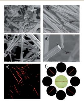
Fig. 1 SEM images of PDI. (a) The solvent was evaporated in vacuum, (b) the solvent was naturally evaporated in several hours, (c) and (d) the solvent was slowly evaporated in several days, (e) PDI rods under cross-polarized microscope, (f) consecutive rotation of a single PDI rod showed alternate appearance of birefringence as the rod was aligned at 45° to the polarizer.
