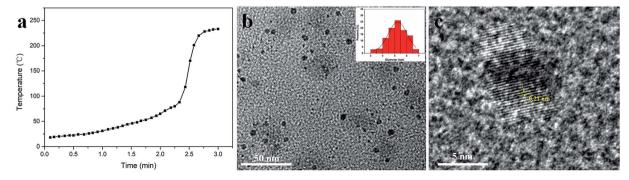
Fig. 2 (a) Relationship between the temperature and the time. Data were obtained per five seconds. (b) A TEM image of the N-CDs. Inset: size distribution. (c) High-resolution TEM image of the N-CDs, and lattice fringes of a single N-CD.
