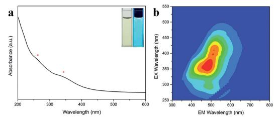
Fig. 4 (a) UV-Vis absorption spectrum of the N-CDs. \*Two absorbance bands at 260 and 340 nm. Inset: images of the N-CD solution in daylight (left) and under 365 nm UV light (right). (b) The 3D fluorescence spectrogram of the N-CDs. Fluorescence intensity increased with color change from blue to red.
