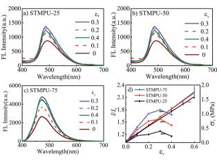
Fig. 2 Fluorescence emission spectra of (a) STMPU-25, (b) STMPU-50 and (c) STMPU-75 films at different tensile strains; (d) true stress—strain curves and fluorescence peak intensity-true strain curves of three AEE polyurethanes.
