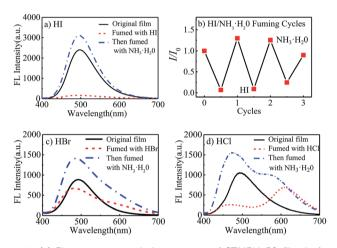
Fig. 3 (a) Fluorescence emission spectra of STMPU-50 film before and after fumed with hydroiodic acid and then fumed with NH $_3\cdot$ H $_2$ O; (b) the quenching and recovery test by HI–NH $_3\cdot$ H $_2$ O fuming cycles; fluorescence emission spectra of STMPU-50 film before and after fumed with (c) hydrobromic acid and (d) hydrochloric acid, and then fumed with NH $_3\cdot$ H $_2$ O.
