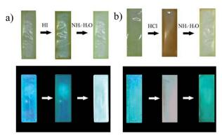
Fig. 4 (a) Color changes of the STMPU-50 film before and after fumed with hydroiodic acid and then smoked with  $NH_3\cdot H_2O$  under normal light (top) and fluorescent changes upon irradiation by 365 nm ultraviolet lamp (bottom); (b) color changes of the STMPU-50 film before and after fumigated with hydrochloric acid and then fumed with  $NH_3\cdot H_2O$  under normal light (top) and fluorescence changes upon irradiation by 365 nm ultraviolet lamp (bottom).
