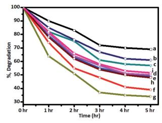
Fig. 9 Degradation of spent wash solution after irradiation with sunlight using (a) undoped TiO<sub>2</sub>, (b) P-25 Degussa, and (c) 1%, (d) 2%, (e) 3%, (f) 4%, (g) 5%, (h) 6%, and (i) 7% Cr-TiO<sub>2</sub> catalysts.
