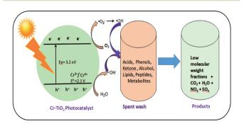
Fig. 10 Scheme of photocatalytic degradation of spent wash solution using  $Cr-TiO_2$  under natural sunlight.
