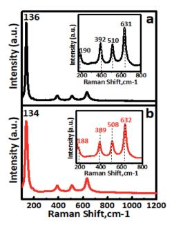
Fig. 5 Room-temperature Raman spectra of (a) undoped  $TiO_2$  and (b) 5%  $Cr-TiO_2$  samples. Inset shows wavenumber shifting.
