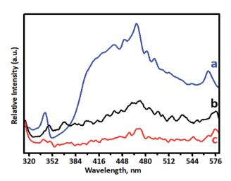
Fig. 7 Photoluminescence spectra of (a) undoped  $TiO_2$ , (b) 1% Cr $-TiO_2$ , and (c) 5% Cr $-TiO_2$ .
