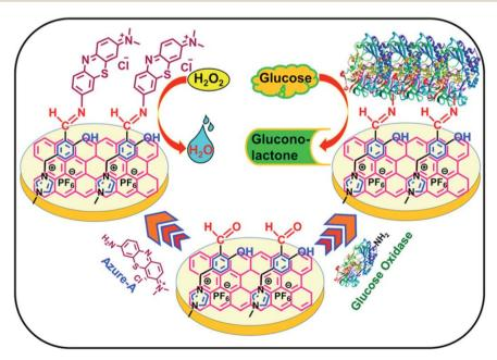
Fig. 6 Schematic illustration of the covalent immobilization of Azure A and GOx on the CHO-IL/EC-rGO/SPE platform. [Reprinted with permission from ref. 199, D. Manoj, K. Theyagarajan, D. Saravanakumar, S. Senthilkumar and K. Thenmozhi, Aldehyde Functionalized Ionic Liquid on Electrochemically Reduced Graphene Oxide as a Versatile Platform for Covalent Immobilization of Biomolecules and Biosensing, *Biosens. Bioelectron.*, 2018, 103, 104–112. Copyright© Elsevier.]
