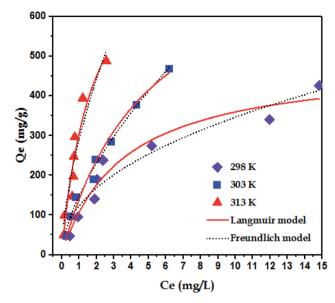
Fig. 6 Nonlinear isotherm models of paraquat adsorbed onto JS/  $\ensuremath{\mathsf{HSO}}\xspace-700.$
