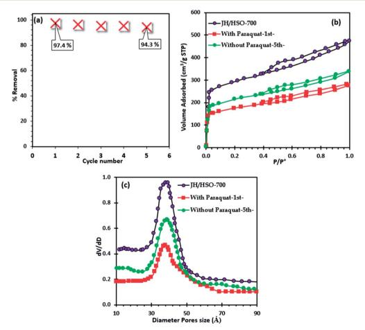
Fig. 7 (a) Regeneration of JS/HSO-700, (b) nitrogen physisorption of JS/HSO-700 after paraguat adsorption and (c) pore size distribution.
