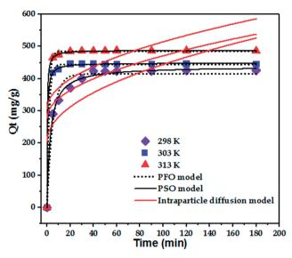
Fig. 5 Nonlinear fit models: PFO, PSO, and IPD
