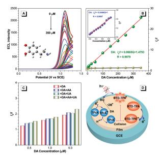
Fig. 5 (A) ECL intensity versus potential profiles of BTD-TPA film with different concentrations of DA. (B) Stern-Volmer plots of  $I_0/I$  of **BTD-TPA** film versus the concentration of DA, AA, and UA. Inset: Stern-Volmer plot at low concentration of DA (0-1  $\mu$ M). (C)  $I_0/I$  of **BTD-TPA** film with different concentrations of DA containing 100-fold concentrations of AA and UA. (D) Proposed ECL quenching mechanism of the BTD-TPA film modified GCE.
