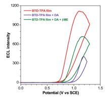
Fig. 6 ECL curves of the BTD-TPA film (red line), +5  $\mu$ M DA (violet line) and +100  $\mu$ M  $\beta$ ME (green line).
