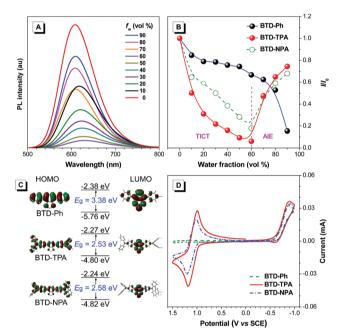
Fig. 2 (A) PL spectra of BTD-TPA in THF/water mixtures with different water fractions  $(f_w)$ . (B) Plots of the relative PL intensity  $(I/I_0)$  versus the composition of the THF/water mixtures of BTD-Ph, BTD-TPA, and BTD-NPA. Io denotes emission intensity in pure THF. Concentration: 10 μM. (C) Optimized geometries and molecular orbitals of HOMO and LUMO levels of the molecules. (D) CVs of BTD-Ph, BTD-TPA, and BTD-NPA in anhydrous DCM.
