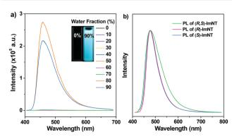
Fig. 2 (a) PL spectra of the dilute solutions of (S)-ImNT in water/THF mixtures with different water fractions ( $f_{\rm w}$ ) (concentration: 0.1 mM). The insets depict the emission images of (S)-ImNT in pure THF and in water/ THF mixtures with 90% water fraction under the illumination of 365 nm UV light. (b) PL spectra of the compounds in the solid state under ambient conditions
