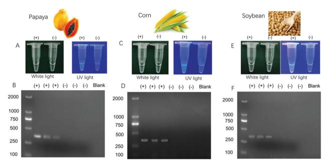
Fig. 3 The visual discrimination results by DNA-binding AIEgens (A, C and E) and results after agarose gel electrophoresis for transgenic and non-transgenic papaya (A and B), corn (C and D) and soybean (E and F). " +" represents three parallel transgenic samples, "-" represents three parallel non-transgenic samples. The expected fragments for papaya, corn and soybean were 369 bp, 333 bp, and 333 bp respectively.
