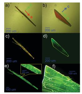
Fig. 1 Optical images of BFMPT single crystals. In transmitted light: form I (a) and form II (b); under blue laser irradiation (405 nm): form I (c) and form II (d), (e) form I after heating at 280 °C for 5 seconds and (f) form II after heating at 280 °C for 5 seconds.
