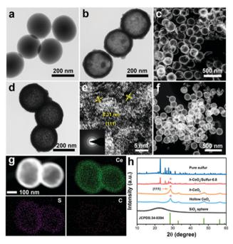
Fig. 2 TEM images of (a) SiO<sub>2</sub> and (b) hollow CeO<sub>2</sub>. (c) SEM image of hollow CeO2. (d) TEM image and (e) HRTEM image of h-CeO2 (the inset shows a SAED pattern). (f) HAADF-TEM image and (g) EDS elemental mapping of h-CeO<sub>2</sub>/sulfur-0.8. (h) XRD patterns.
