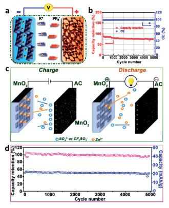
Fig. 9 (a) Schematic and (b) long-term cycling stability at the current density of 1 A g<sup>-1</sup> of a NGC//KTO KIHSCD (modified from ref. 125, copyright permission from the American Chemical Society); (c) schematic illustration and (d) cycling stability of a designed MnO<sub>2</sub>//AC ZIHSCD (modified from ref. 126, copyright permission from Elsevier).
