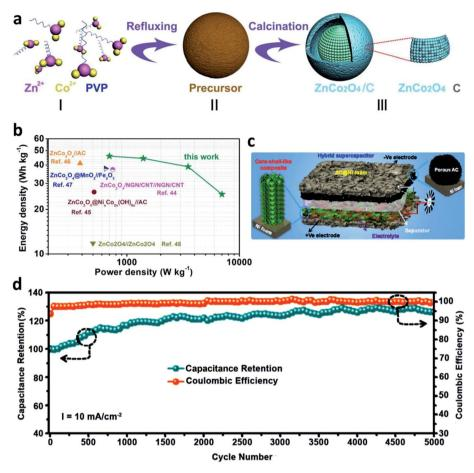
Fig. 4 (a) Scheme of the synthesis a yolk–shell structure ZnCo<sub>2</sub>O<sub>4</sub> material, (b) Ragone plots of AACSDs (modified from ref. 85, copyright permission from the Royal Society of Chemistry); (c) illustration for the preparation process and (d) cycling stability of core-shell-like NiO@Co<sub>3</sub>O<sub>4</sub>-NiO FTN/Ni foam (modified from ref. 88, copyright permission from Elsevier).
