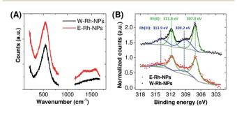
Fig. 2 (A) Raman spectra of Rh NPs obtained in water or ethanol. (B) Xray photoelectron spectroscopy (XPS) spectra of Rh NPs E-Rh/C and W-Rh/C inks obtained in different liquid environments.
