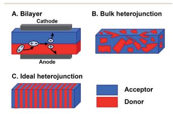
Fig. 1 Donor-acceptor heterojunction morphologies. (A) Bilayer structure showing process of charge collection in OPV devices. (B) Bulk heterojunction (BHJ) and (C) heterojunction optimized to increase junction area, while providing contiguous pathways for charges to migrate to the electrodes.
