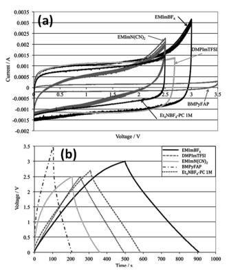
Fig. 18 (a) CV of various electrolytes at 5 mV  $s^{-1}$  and (b) galvanostatic charge-discharge at 2 mA cm<sup>-2</sup>. This figure has been adapted from ref. 168 with permission from the Royal Society of Chemistry.
