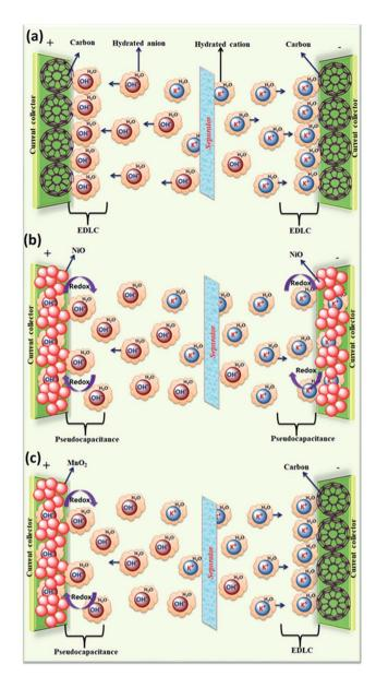
Fig. 6 Graphical representation of reaction mechanism between alkaline electrolyte (KOH) and carbon– $MnO_2$  electrodes for (a) EDLC (b) pseudocapacitor (c) hybrid supercapacitor.
