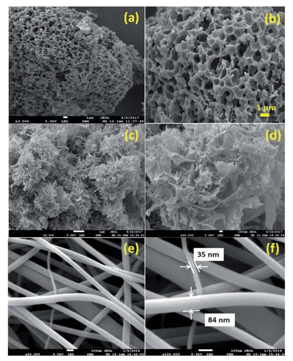
Fig. 24 FE-SEM images of various electrode materials: (a and b) porous carbon, (c and d) SnO<sub>2</sub>/TiO<sub>2</sub> composite flowers and (e and f) Cu<sub>2</sub>O nanowires. (a and b) have been adapted from ref. 81 with permission from Elsevier. (c and d) have been adapted from ref. 180 and (e and f) have been adapted from ref. 29 with permission from the American Chemical Society.
