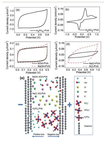
Fig. 20 CV curves of the as-prepared solid-state supercapacitors with different electrolytes at 100 mV s $^{-1}$  scan rate. (a)  $\rm H_3PO_4-PVA$  and (b)  $\rm H_2SO_4-PVA$  electrolyte. (c) Base gel electrolytes: KOH (black) and NaOH (red dashed) and (d) neutral gel electrolytes: NaCl (black) and KCl (red dashed). (e) Schematic illustration of ion diffusion in different electrolytes. This figure has been adapted from ref. 204 with permission from the Royal Society of Chemistry.
