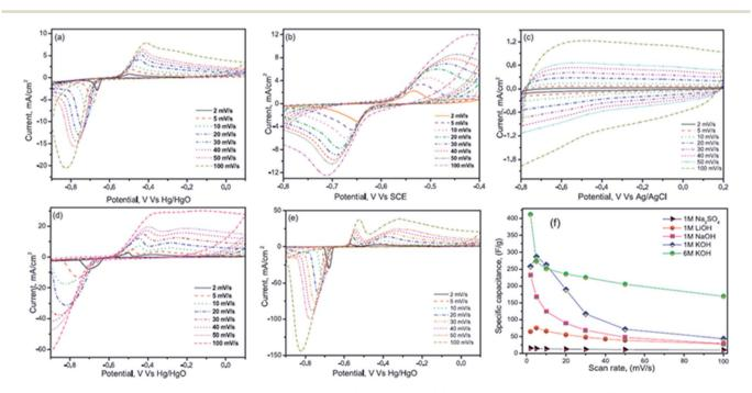
Fig. 9 CV curves at various scan rates of (a) 1 M LiOH (b) 1 M NaOH (c) 1 M Na<sub>2</sub>SO<sub>4</sub> (d) 1 M KOH and (e) 6 M KOH and (f) capacitance vs. scan rate for different electrolytes. This figure has been adapted from ref. 116 with permission from Elsevier.
