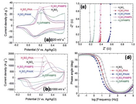
Fig. 21 CV of the ePAn electrode for the supercapacitor adopting  $H_2SO_4$ ,  $H_2O/PAMPS$ ,  $H_2SO_4/PAA$ , and  $H_2SO_4/PAA$  as the electrolyte system, at scan rates of (a) 20 and (b) 1000 mV s<sup>-1</sup>. (c) Nyquist and (d) Bode plots for the ePAn electrode for the supercapacitor adopting various acrylic gel polymer electrolytes. This figure has been adapted from ref. 206 with permission from Elsevier.
