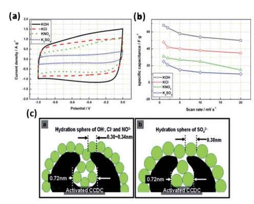
Fig. 8 (a) Cyclic voltammograms of activated CCDC supercapacitors in the aqueous electrolytes 0.5 M K<sub>2</sub>SO<sub>4</sub>, 2 M KCl, 1 M KNO<sub>3</sub> and 6 M KOH  $(20 \text{ mV s}^{-1})$  and (b) the specific capacitance of the supercapacitor at different scan rates. (c) Schematic diagram of the relationship of hydration sphere ions and pores. This figure has been adapted from ref. 115 with permission from Elsevier.
