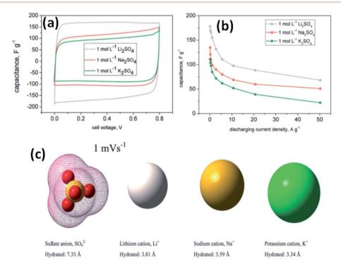
Fig. 11 (a) CV curves of a carbon based supercapacitor in 1 mol  $L^{-1}$  alkali metal sulfate solutions (Li, Na, K) at 1 mV s<sup>-1</sup>, (b) capacitance vs. current load for different alkali metal sulfates solutions, and (c) ion shape and dimensions in aqueous solutions. This figure has been adapted from ref. 118 with permission from the Royal Society of Chemistry.
