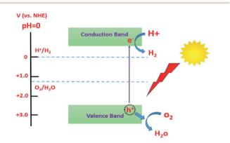
Fig. 9 Semiconductor requirements for solar water splitting
