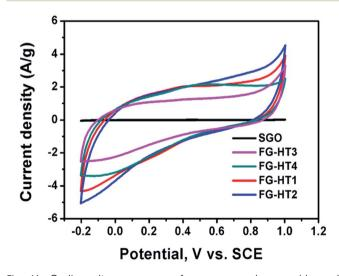
Fig. 11 Cyclic voltammograms of spongy graphene oxide and hydrogenated  ${\rm TiO_2}$  with different ratios of functionalized graphene oxide. Reproduced from ref. 117 with permission from the Royal Society of Chemistry.
