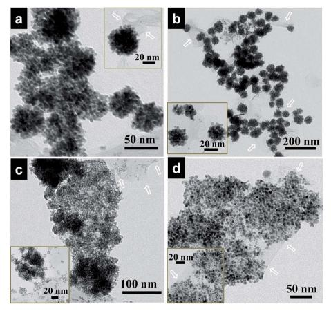
Fig. 2 TEM images of Pd-Fe nanoalloys deposited on graphitic carbon nanosheets. (a) Pd<sub>96</sub>Fe<sub>4</sub>/GCN, (b) Pd<sub>91</sub>Fe<sub>9</sub>/GCN, (c) Pd<sub>85</sub>Fe<sub>15</sub>/GCN, and (d) Pd<sub>77</sub>Fe<sub>23</sub>/GCN nanohybrids. Inset: the corresponding Pd–Fe nanoalloys at high magnification. The white arrows represent the thin sheets of graphitic carbon.
