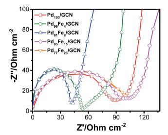
Fig. 6 Nyquist plots of the  $Pd_{100}/GCN$ ,  $Pd_{96}Fe_4/GCN$ ,  $Pd_{91}Fe_9/GCN$ ,  $Pd_{85}Fe_{15}/GCN$  and  $Pd_{77}Fe_{23}/GC$  nanohybrids. Nyquist plot analysis indicates that the  $Pd_{96}Fe_4/GCN$  anode with small charge transfer resistance would be an outstanding anode material for DAFCs.
