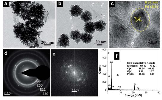
$\textbf{Fig. 1} \quad (a \text{ and b}) \ Transmission \ electron \ micrographs \ of \ the \ Pd_{100}/GCN \ nanohybrid \ at \ two \ different \ magnifications, \ (c) \ HRTEM \ image \ of \ palladium \ descriptions \ descriptions$ nanoparticles, (d) SAED pattern and (e) FFT and (f) EDS spectrum of the Pd<sub>100</sub>/GCN nanohybrid. The white arrows represent the thin sheets of graphitic carbon.
