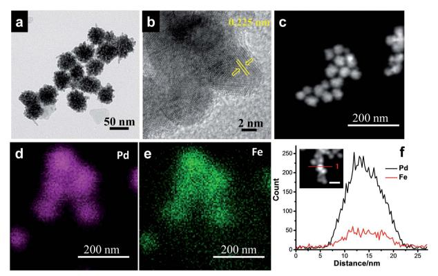
Fig. 3 (a) TEM, (b) HRTEM, and (c) HAADF-STEM images, and (d and e) elemental mapping and (f) EDS line scanning profiles of the Pd<sub>91</sub>Fe<sub>9</sub>/GCN nanohybrids.
