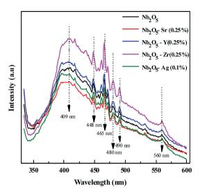
Fig. 5 PL spectra of the doped and pristine Nb<sub>2</sub>O<sub>5</sub>.
