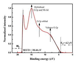
Fig. 4 UPS spectra of Nb<sub>2</sub>O<sub>5</sub>
