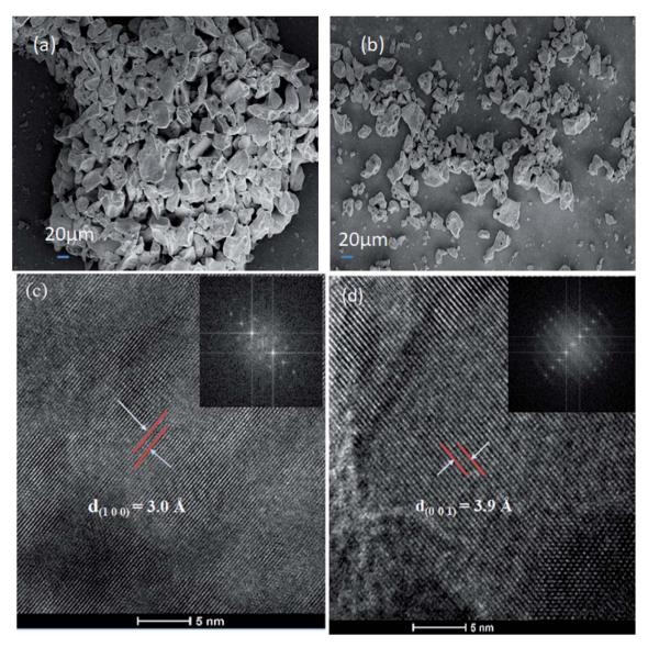
Fig. 7 (a) SEM image of Nb<sub>2</sub>O<sub>5</sub>, (b) SEM image of Sr (0.25%)–Nb<sub>2</sub>O<sub>5</sub>, (c) HRTEM image of Nb<sub>2</sub>O<sub>5</sub> showing the *d* spacing of the (100) plane and the inset shows the FFT image, and (d) HRTEM image of Nb<sub>2</sub>O<sub>5</sub> showing the *d* spacing of the (001) plane and the inset presents the FFT image.
