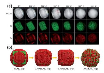
Fig. 4 (a) Surface transformation, atomic redistribution and alloying process of Au@Pd core-shell NPs in TEM observation. (b) Atomic KMC simulations of the Pd@Au NP transformation process from a coreshell structure to mixed alloys at 600 °C. Adapted with permission from ref. 59. Copyright 2019 The Royal Society of Chemistry.
