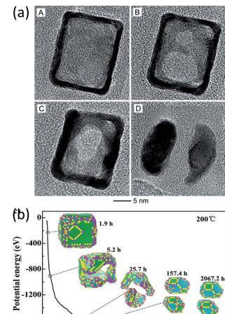
Fig. 5 (a) TEM images of a Pt hollow nanocube disintegrating at elevated temperature. Adapted with permission from ref. 60. Copyright 2018 Wiley-VCH Verlag GmbH & Co. KGaA, Weinheim. (b) Structure evolution simulation of a Pt hollow nanocube at 200 °C. Adapted with permission from ref. 38. Copyright 2018 Wiley-VCH Verlag GmbH & Co. KGaA, Weinheim.
