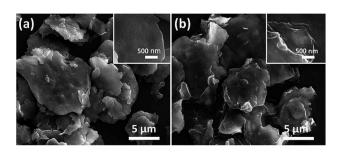
Fig. 10 (a) SEM images of FCI and (b) RGO-coated FCI $^{66}$  – reproduced by permission of the Royal Society of Chemistry.
