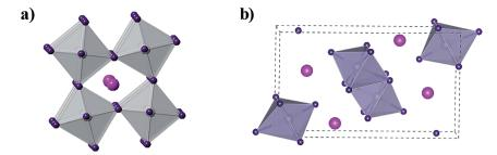
Fig. 6 (a) Crystal structure of  $B-\gamma-CsSnl_3$ . B(b) Crystal structure of Y-CsSnl<sub>3</sub>. In these two images, the magenta spheres represent the Cs atoms, the purple spheres represent the I atoms, and the gray spheres represent the Sn atoms.
