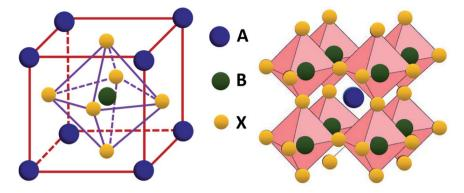
Fig. 3 Structure of perovskites with ABX<sub>3</sub> formula
