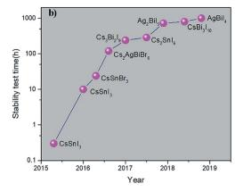
Fig. 2 (a) Highest PCE of devices based on different inorganic lead-free perovskite materials reported to date (classified by element). (b) Stability test time evolution of inorganic lead-free perovskites.
