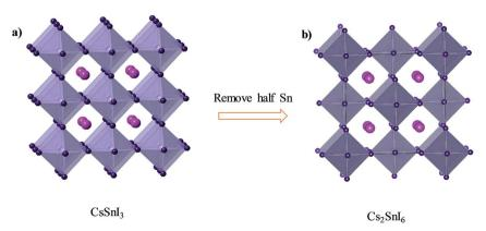
(a) Crystal structure of CsSnl<sub>3</sub>. (b) Crystal structure of Cs<sub>2</sub>Snl<sub>6</sub>. Consulting from ref. 79.
