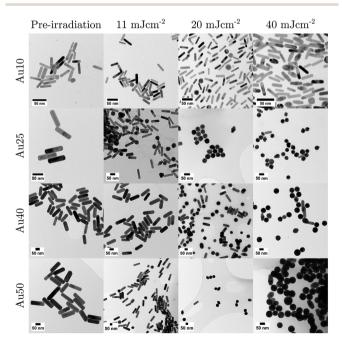
Fig. 4 TEM images taken for each sized AuNR at specific points in the study: before laser irradiation, and after 20 pulses at  $11 \text{ mJ cm}^{-2}$ ,  $20 \text{ mJ cm}^{-2}$ , and  $40 \text{ mJ cm}^{-2}$ . Scale bars = 50 nm.
