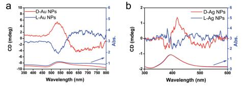
Fig. 6 CD and UV-vis spectra of (a) chiral Au NPs and (b) Ag NPs dispersed in water obtained from the hydrolysis (by using 5 wt% NaOH) of chiral Au@SiO<sub>2</sub>-500 and Ag@SiO<sub>2</sub>-600, respectively.
