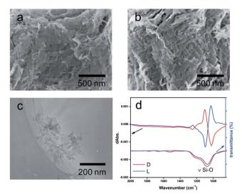
Fig. 1 SEM images of calcined silicas, (a) D-SiO<sub>2</sub>-600 and (b) L-SiO<sub>2</sub>-600. TEM images of (c) the piece of L-SiO<sub>2</sub> crushed by homogenizing the methanol solution containing chiral silica bundles (calcined PEI/ tart@SiO<sub>2</sub>) for at least 20 000 rpm for 2 min. (d) FT-IR/VCD spectra of the crushed SiO<sub>2</sub>, red lines for the D-form, and blue lines for the L-form.
