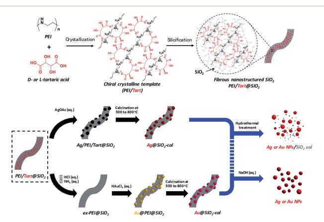
Scheme 1 Representation of the procedure for obtaining chiral SiO<sub>2</sub> and metal@SiO<sub>2</sub> composites and two approaches for isolation of metal NPs from the metal@SiO2 composites.
