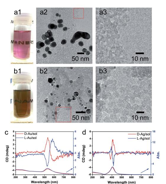
Fig. 4 Aqueous solution of L-Au/sol (a1) and L-Ag/sol (b1). TEM images at different magnifications of L-Au/sol (a2 and a3) and L-Ag/sol (b2 and b3) (taken from a highly diluted solution containing Au/sol or Ag/sol). CD and UV-vis spectra of Au/sol (c) and Ag/sol (d) (both samples were diluted from their stock solutions), red lines for the p-form and blue lines for the p-form.
