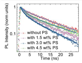
Fig. 6 The time resolved PL demonstrates the reduced exciton quenching lifetime without PS and with 1.5 wt%, 3.0 wt%, and 4.5 wt%
