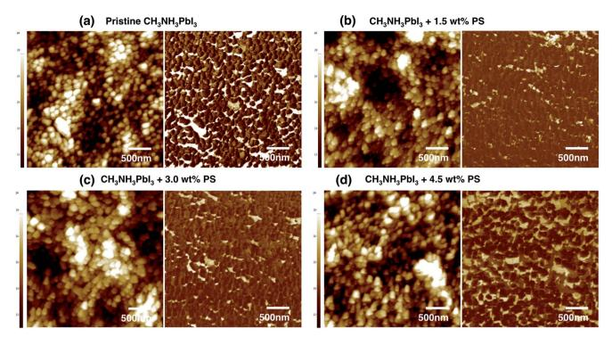
Fig. 3 Surface properties of thin films used in this work. The (a-d left panels) atomic force microscopy (AFM) and (a-d right panels) conductive AFM (cAFM) images of CH<sub>3</sub>NH<sub>3</sub>PbI<sub>3</sub> perovskite thin film with different concentrations of polystyrene on the ITO/PEDOT:PSS layer.
