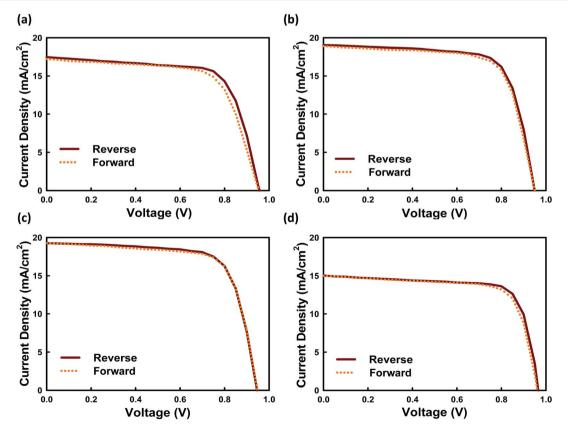
Fig. 7 J-V plots for perovskite solar cells (a) without PS, (b) with 1.5 wt% PS, (c) with 3.0 wt% PS, and (d) with 4.5 wt% PS under one sun conditions (100 mW cm $^{-2}$ , AM1.5G). The scan rate for both scans is 10 mV s $^{-1}$ .
