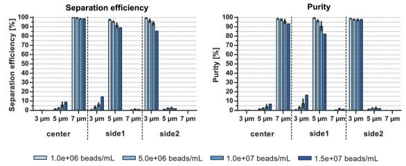
Fig. 5 Particle separation vs. sample bead concentration. Acoustophoretic separation of an equal mixture of 3, 5 and 7 μm polystyrene beads was performed at 500 µL min<sup>-1</sup> sample flow while altering the initial sample concentrations. Shown are the separation efficiency and purity of the different beads in the three outlets (n = 3, mean  $\pm$  SD).
