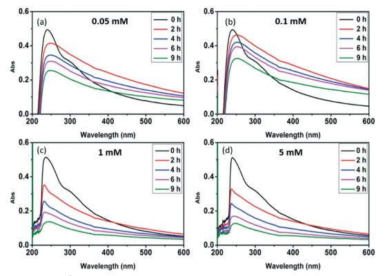
Fig. 3 UV-vis spectra of 10 mg L<sup>-1</sup> GO suspensions before and after UV irradiation in the presence of nitrate at different concentrations (a: 0.05 mM; b: 0.1 mM; c: 1 mM; and d: 5 mM), showing the concentration-dependent effects of nitrate on the structural changes of GO nanosheets. Red shift of  $\lambda_{max}$  of GO suspension was observed at nitrate concentrations of 0.05 and 0.1 mM, whereas blue shift of  $\lambda_{max}$  was observed at nitrate concentrations of 1 and 5 mM.
