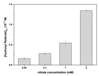
Fig. 5 Production of 'OH under UV irradiation of 10 mg L<sup>-1</sup> GO suspension, as affected by the concentration of nitrate (0.05, 0.1, 1 and 5 mM), showing that the concentration of 'OH was dependent upon the nitrate concentration (the ['OH]ss generated in the system containing only GO was minimal and calibrated to zero).
