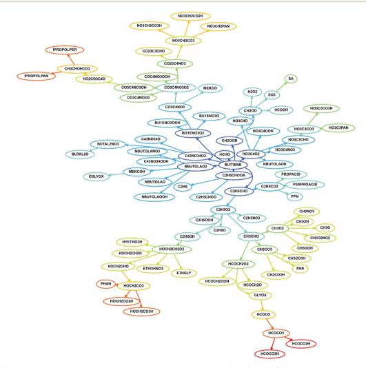
Fig. 1 A simplified representation of the degradation scheme for 1-butene based on MCM chemistry and nomenclature (http://mcm.leeds.ac.uk/MCM/). Note that several of the smaller molecules ( $NO_2$ , CO,  $HO_2$ ,  $HNO_3$ , OH,  $O_3$ ,  $H_2$ ,  $NO_3$ ) have been ignored for simplicity. The different colours represent different oxidation stages. The blues denote the preliminary oxidation steps, with subsequent reaction steps being shown in yellow, orange and red.
