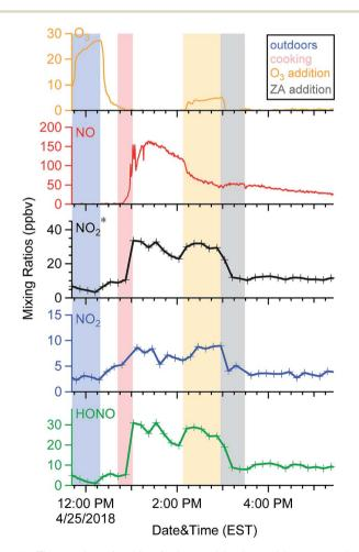
Fig. 6 Time series of oxidant\* observed in the residence sampled through the environmental chamber during an O<sub>3</sub>-perturbation experiment performed after cooking. Shaded areas indicate different conditions noted in the legend of the graph.
