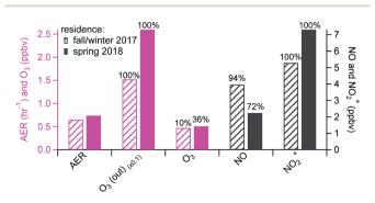
Fig. 2 Average AER, ambient outdoor O<sub>3</sub> levels, and mixing ratios of O<sub>3</sub> and nitrogen oxides in the residence under background conditions in two seasons. Data below the detection limit were included to calculate averages. Text above the bars indicates the percentage of data above the detection limit.
