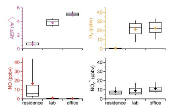
Fig. 1 Statistics of the air exchange rate (AER) and mixing ratios of  $O_3$ , NO, and the sum of  $NO_2$  and HONO ( $NO_2$ \*) observed in three indoor environments in Syracuse, NY, over the entire field study period. The box and whisker plots show the median (line), mean (marker), upper and lower quartiles (box), and the 10th and 90th percentiles (whiskers).
