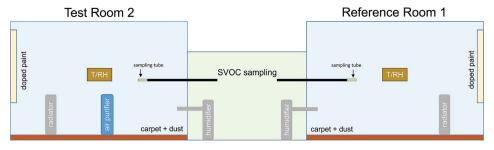
Fig. 1 Design of the test house experiments.
