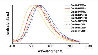
Fig. 10 Emission spectra of PMMA, DPEPO and mCBP films with 10 wt% of the complexes Cu-1b, Cu-2b and Cu-2c respectively, measured at room temperature with 350 nm excitation wavelength.
