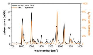
**Fig. 14** Excited state spectrum (black) and calculated  $T_1$  spectrum (orange) (B3LYP-D3(BJ)/def2-TZVP, FWHM = 8 cm $^{-1}$ , Gaussian profile, scaled by 0.975) of **Cu-2b**. The  $T_1$  specific bands are marked with asterisks.
