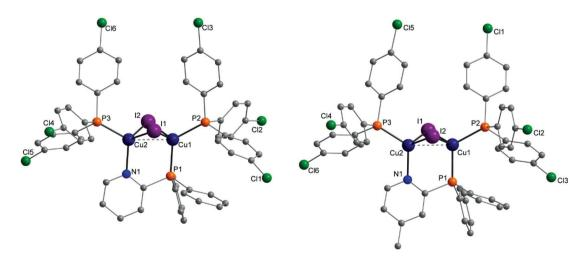
Fig. 4 Molecular structures of complexes Cu-1d and Cu-2d bearing tris(4-chlorophenyl)phosphine as ancillary ligands. Hydrogen atoms and solvent molecules were omitted for clarity.
