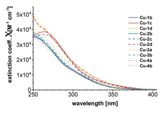
Fig. 5 Absorption spectra of all copper complexes Cu-1b–Cu-4b measured in DCM (7  $\times$  10<sup>-6</sup> M) at room temperature.
