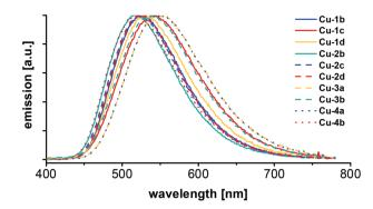
Fig. 8 Emission spectra of the series of Cu(ı) AlkylPyrPhos complexes, measured of the powder samples at room temperature with 350 nm excitation wavelength.
