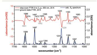
Fig. 13 FTIR ground state spectrum at 20 K (black), calculated So spectrum (B3LYP-D3(BJ)/def2-TZVP, FWHM = 8 cm<sup>-1</sup>, Gaussian profile, scaled by 0.975) (blue) and step-scan difference spectrum 0 to 2 µs after excitation ( $\lambda_{EX}$  = 355 nm) (red) of Cu-2b.
