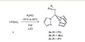
Scheme 1 Synthesis of 2a-c (R = Ph, nBu, iPr).
